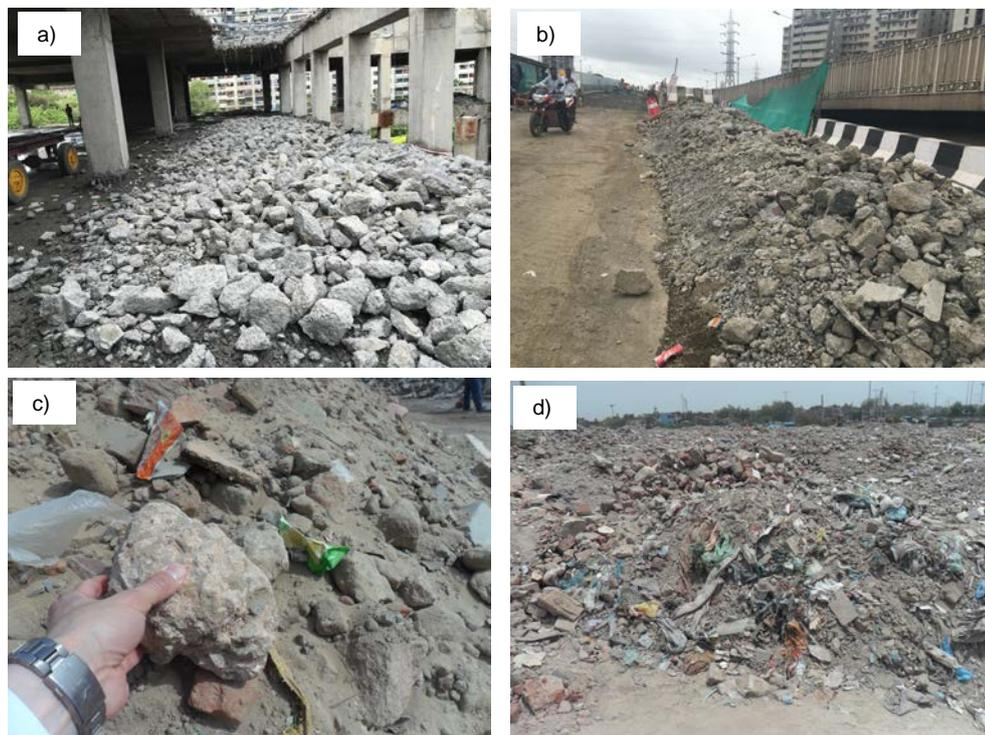
**Fig-1: Different C&D waste from a) Office building in Mumbai b) Reconstruction of Amar Mahal flyover in Mumbai c) feedstock material to Burari recycling facility in Delhi d) mixed waste at collection site in Delhi**
