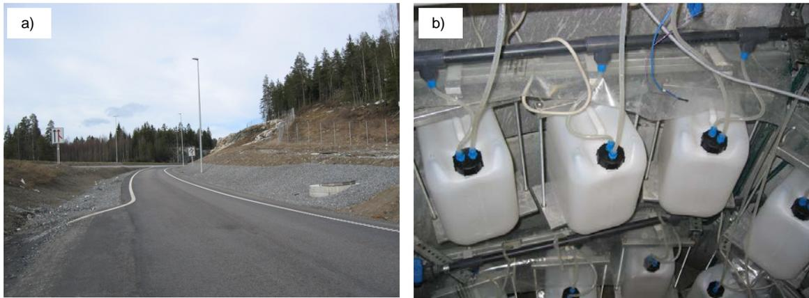
**Fig-4: a) Recycled aggregates with particle size 20/120 mm applied in test segments of the road sub-base in the entrance lane to the north-bound lane of E6 Taraldrud b) Collection of the infiltration water from sub-base were conducted in separate sampling lines inside a collection well**
