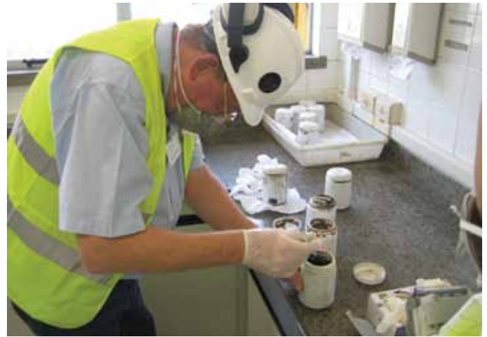
Figure XX.4: sampling and analysis of alternative fuels at the pre-processing facility
