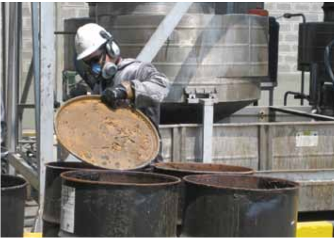
Figure XX.3: inspection of drums with hydrocarbon sludge before pre-processing
